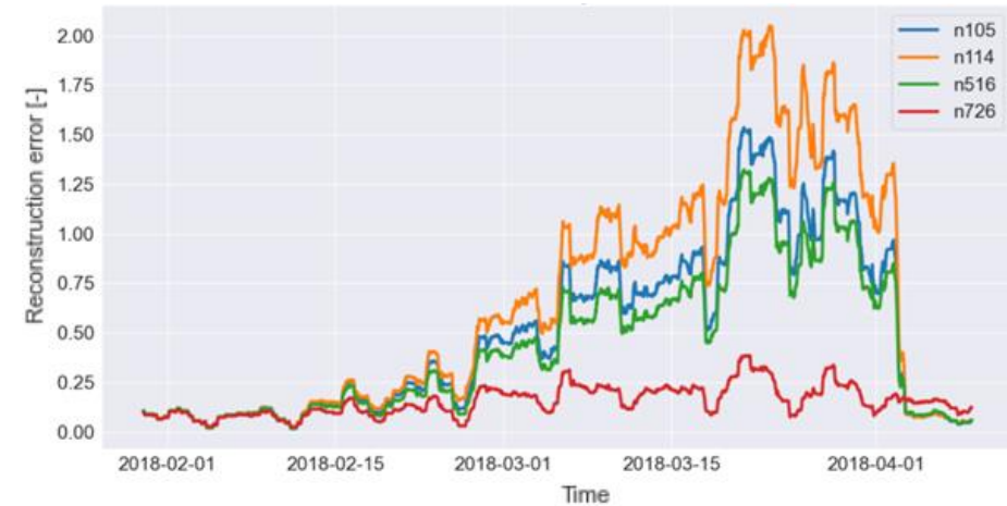
Incipient leak at p461 (4.28 m 3 /hr)
